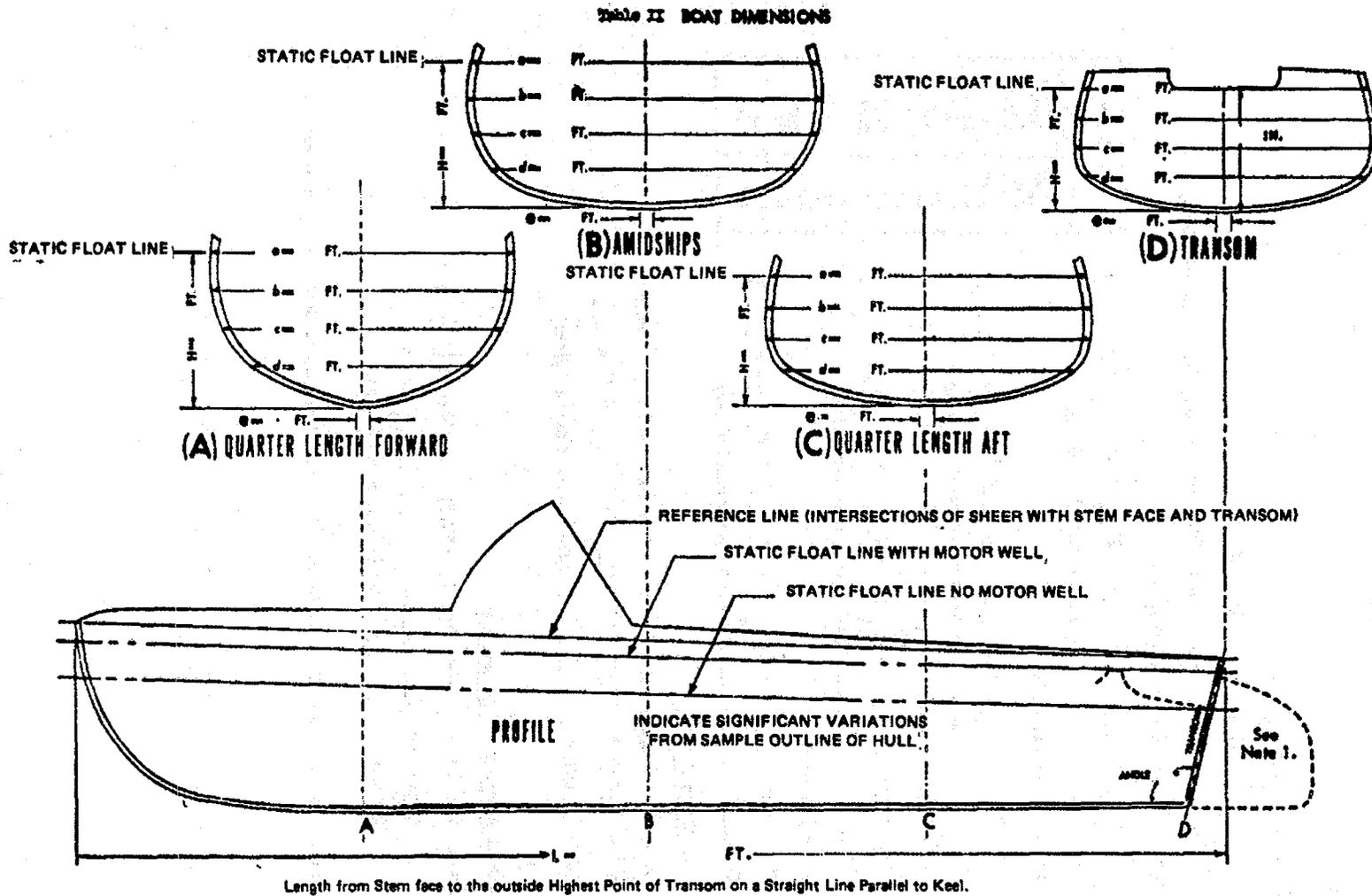
**STATIC FLOAT LINE** passes through the point of major leakage and is parallel with a line connecting the intersections of the sheer with the forward face of the stem and the sheer with the afterface of the transom.
