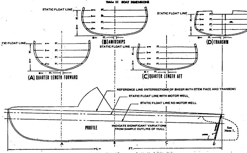
Length from Stem face to the outside Highest Point of Transom on a Straight Line Parallel to Keel.
