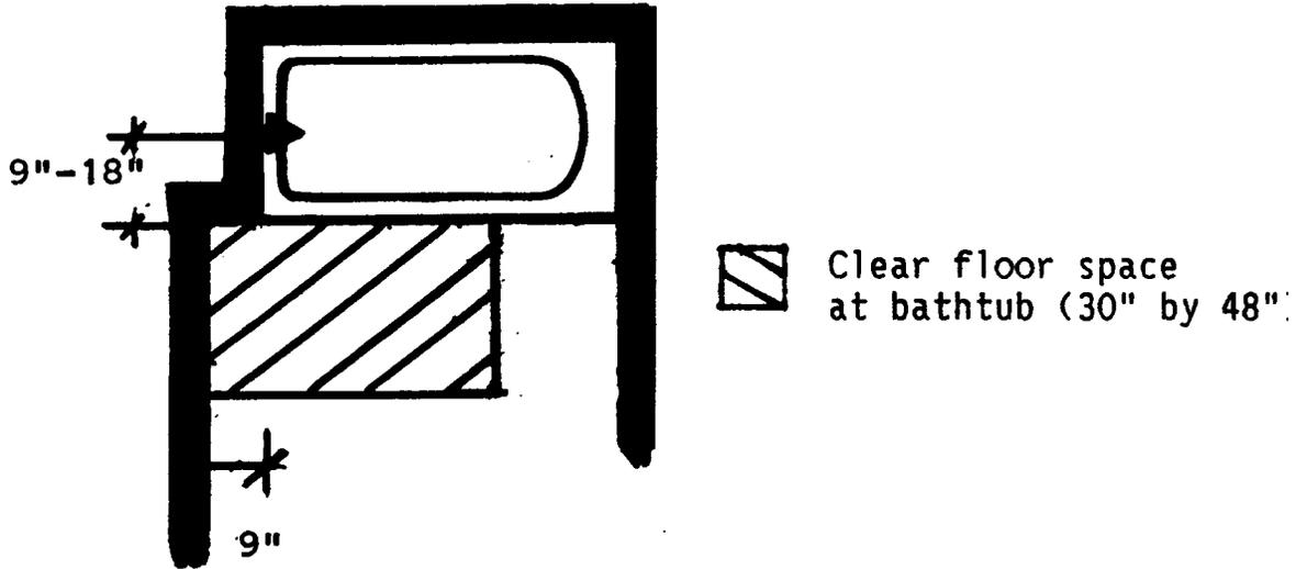
b. Where the centerline of the controls is located between 9 inches and 18 inches from the apron of the bathtub, a clear floor space at least 30 inches by 48 inches shall extend at least 9 inches beyond the head of the bathtub as shown in Figure 57.871-2.
