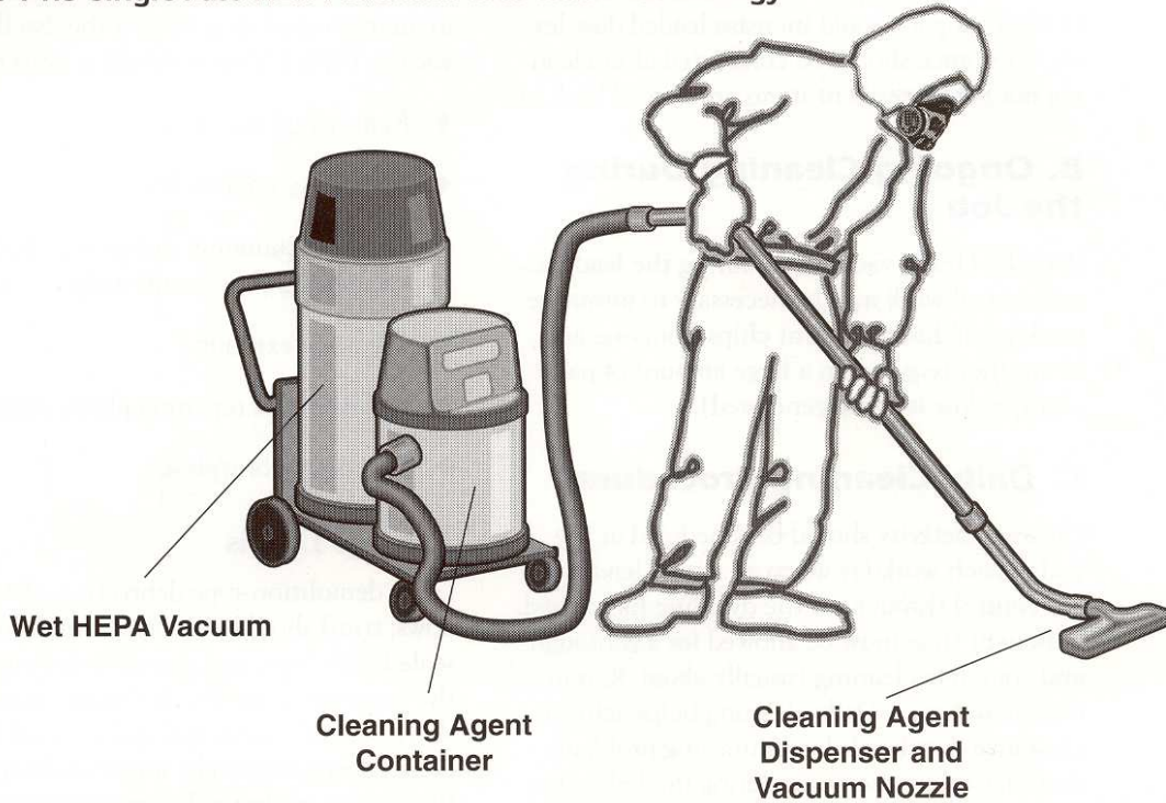
Figure 14.5 Single-Pass HEPA Vacuum/Wet Wash Technology.
