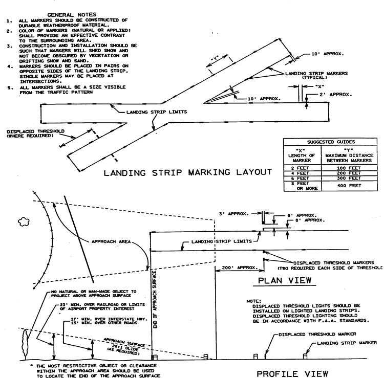
DISPLACED THRESHOLD MARKER LAYOUT
