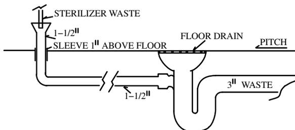
3. Battery assemblies. A battery assembly of not more than 3 sterilizer wastes may drain to one trap, provided the trap and waste are sized according to the combined fixture unit rating; the trap is located immediately below one of the indirect waste connections; the developed distance of a branch does not exceed 8 feet; and the branches change direction through a tee-wye or wye pattern fitting.
