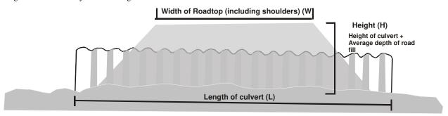
Determining the length of a culvert:
