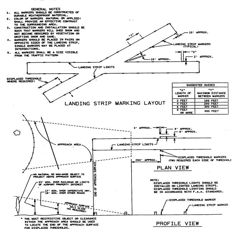
DISPLACED THRESHOLD MARKER LAYOUT
