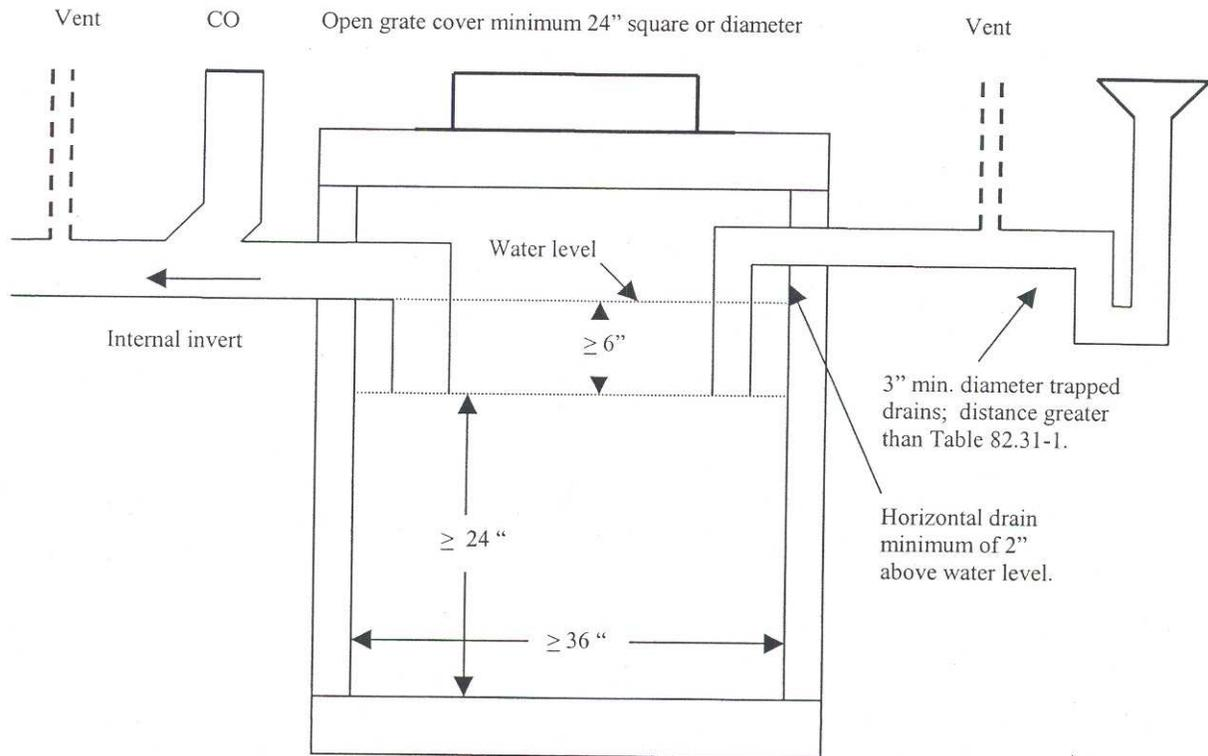
**A-82.34 (4)-3. TRAPPED FIXTURE DISCHARGING INTO GARAGE CATCH BASIN.**
