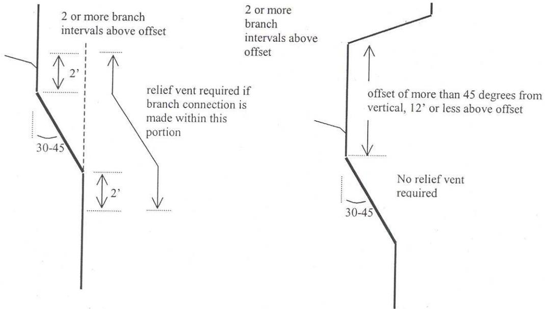
**A-82.31 (5) (b) RELIEF AND YOKE VENTS FOR OFFSETS OF MORE THAN 45 DEGREES.**
