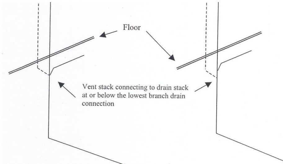
A-82.31 (4)-3. VENT STACKS AND STACK VENTS.
