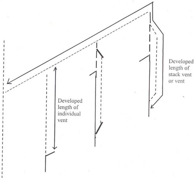
**A-82.31 (14) (c) SIZING BRANCH VENTS SERVING A WET VENT.**
