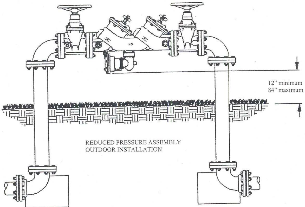
A-82.41 (5) (f)-3. CROSS CONNECTION CONTROL ASSEMBLY INSTALLATION.
