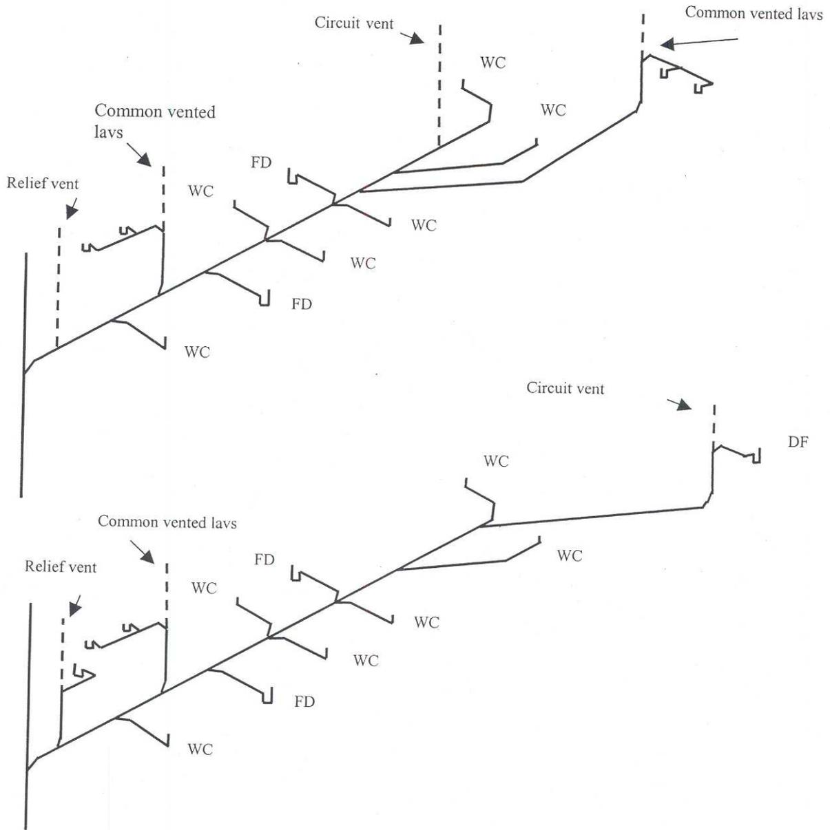
**A-82.31 (1) (a) COMMON VENTS, VERTICAL, SERVING ANY TWO FIXTURES.**
