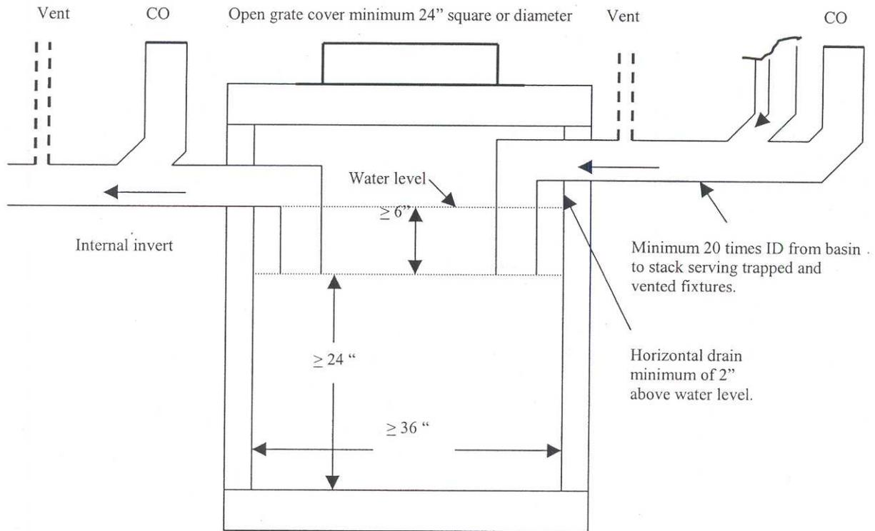
**A-82.34 (4)-6. GARAGE CATCH BASIN RECEIVING PRESSURIZED DRAINS.**
