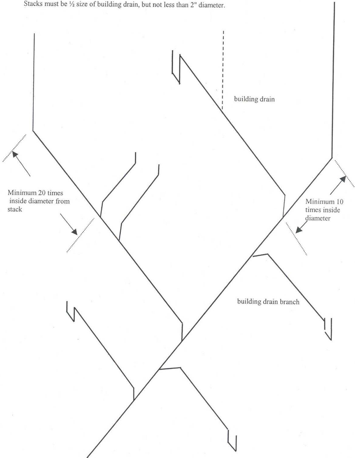
A-82.31 (17) (c) COMBINATION DRAIN AND VENT LABORATORY SINK VENTING.
