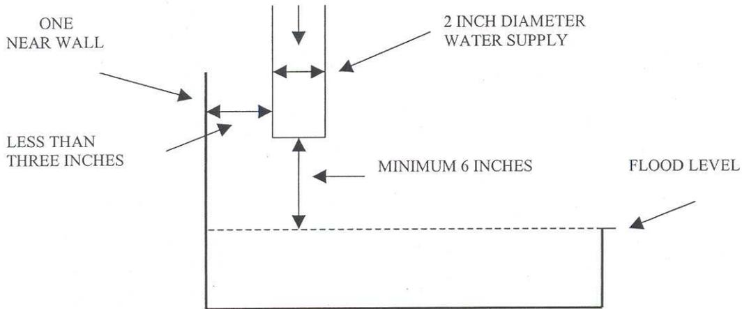
If distance is three times or greater than the diameter of water supply (2 inches) then the air gap is two times the diameter of the water supply, (i.e.,  $2 \times 2 = 4$  inches)
