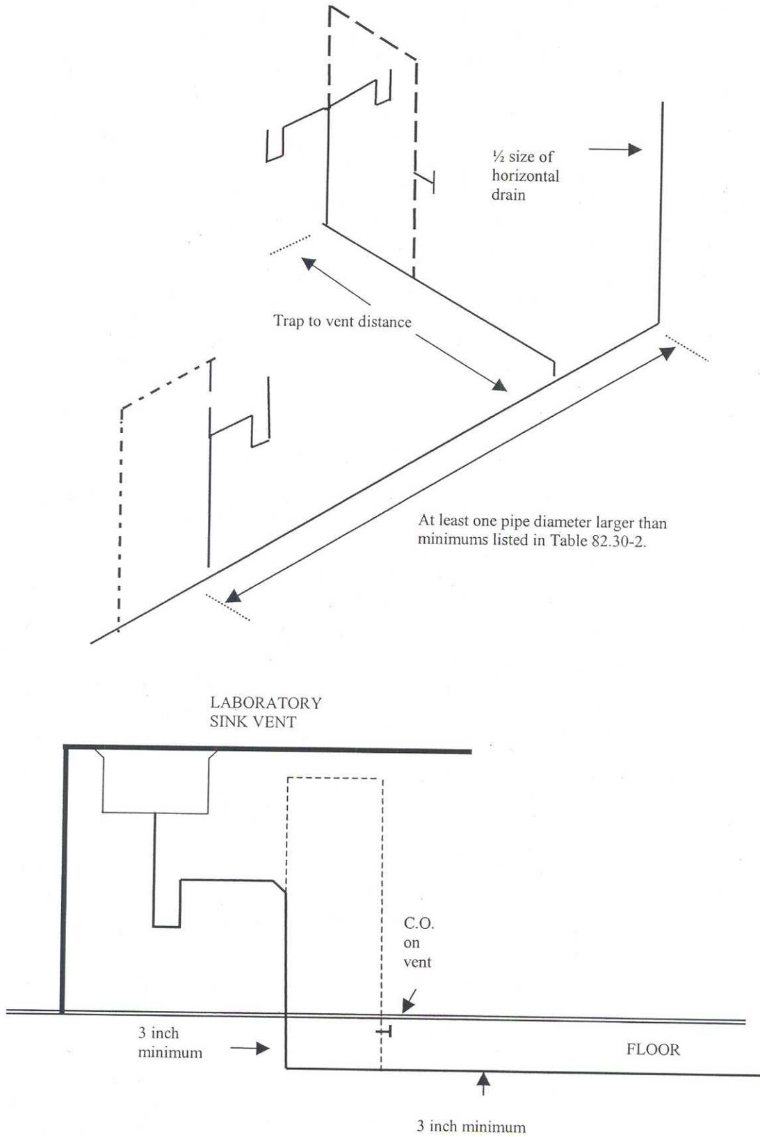
**A-82.32 (4) (b) INSTALLATION OF TRAPS.**
