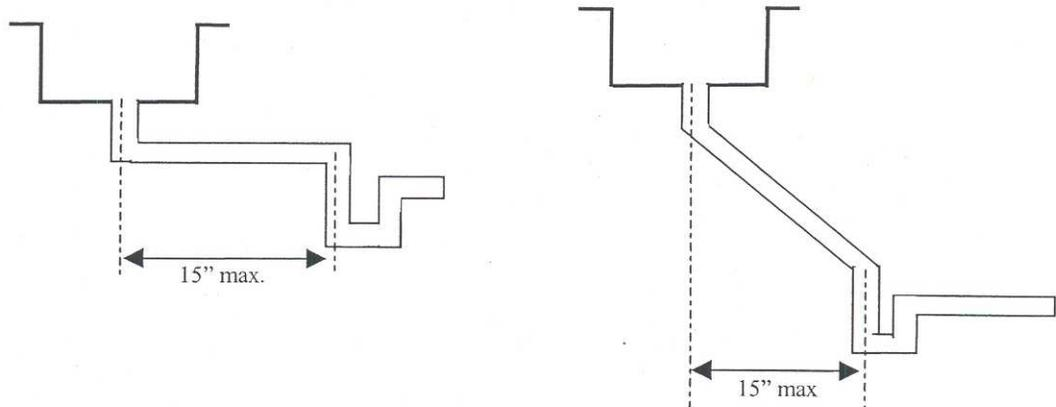
Horizontal distance between fixture drain outlet and trap
