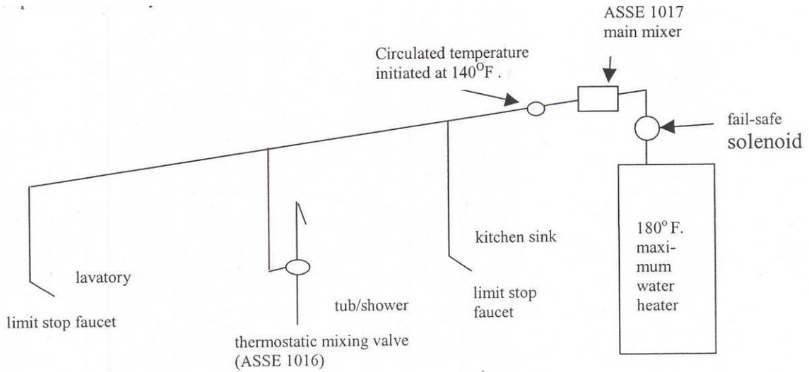
**Option 4.** Fail safe solenoid provided at main mixer meeting ASSE 1017, combination thermostatic/pressure balance mixing valve meeting ASSE 1016 and limit stop faucets at lavatory and kitchen sink.
