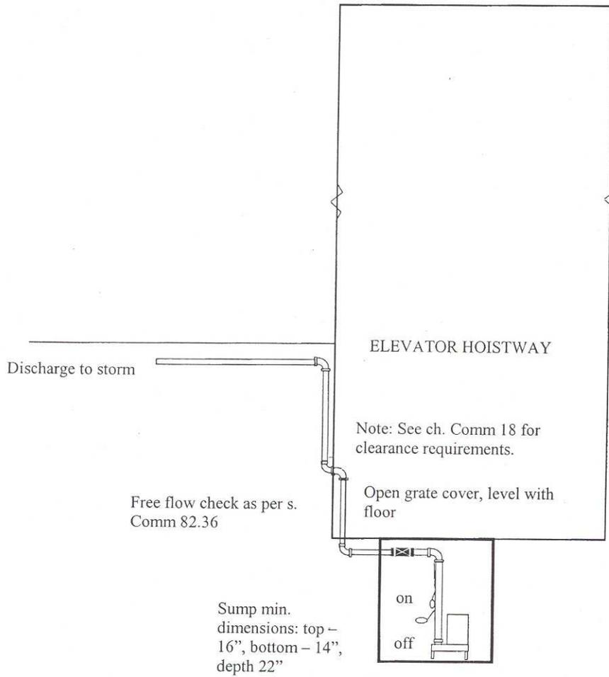
**A-82.33 (9) (f)-2. ELEVATOR PIT SUBSOIL AND FLOOR DRAINS.**
