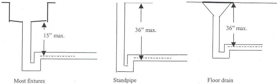
Vertical distance between fixture drain outlet and trap
