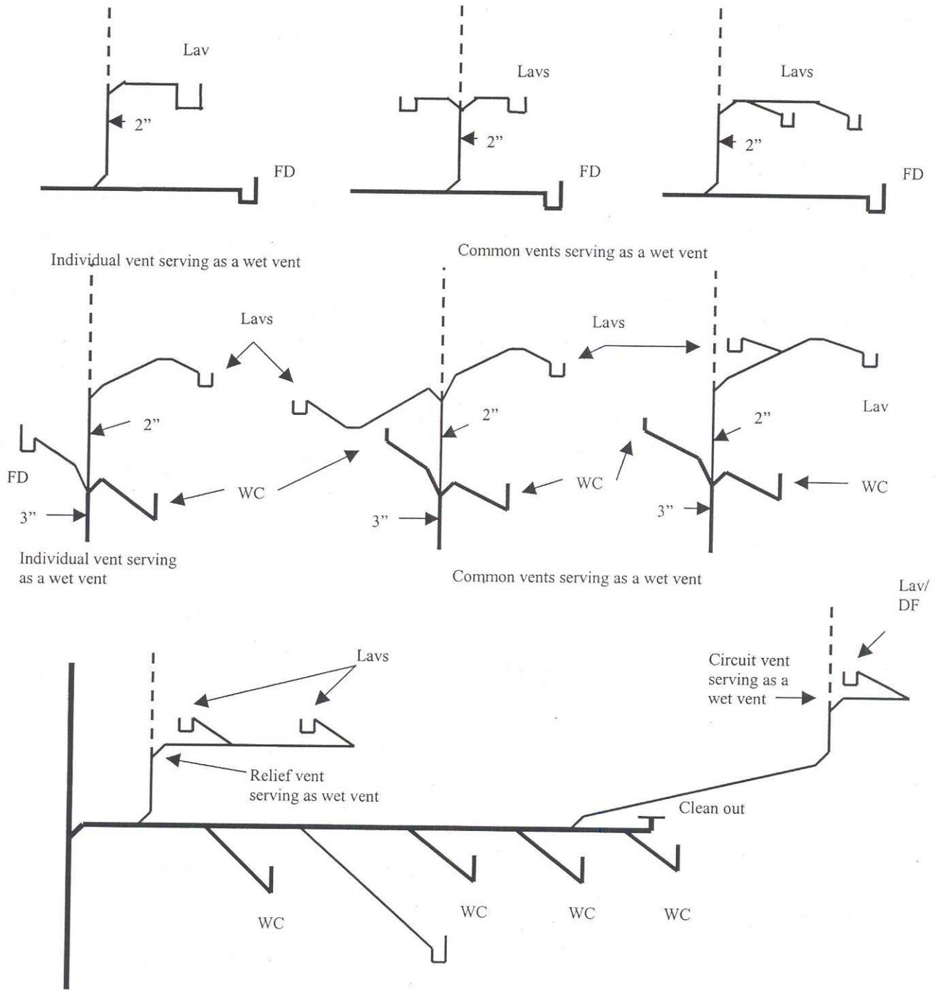
**A-82.31 (14) (a) and (b) SIZING VENT STACKS AND STACK VENTS.**
