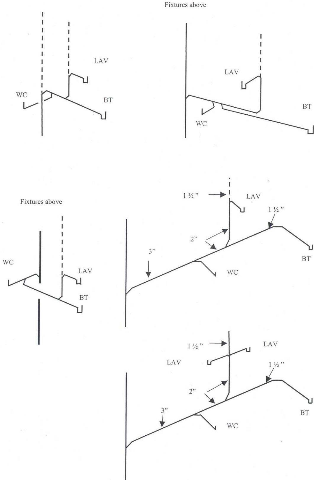
**A-82.31 (13)-2. WET VENTING - FLOOR OUTLET FIXTURES.**
