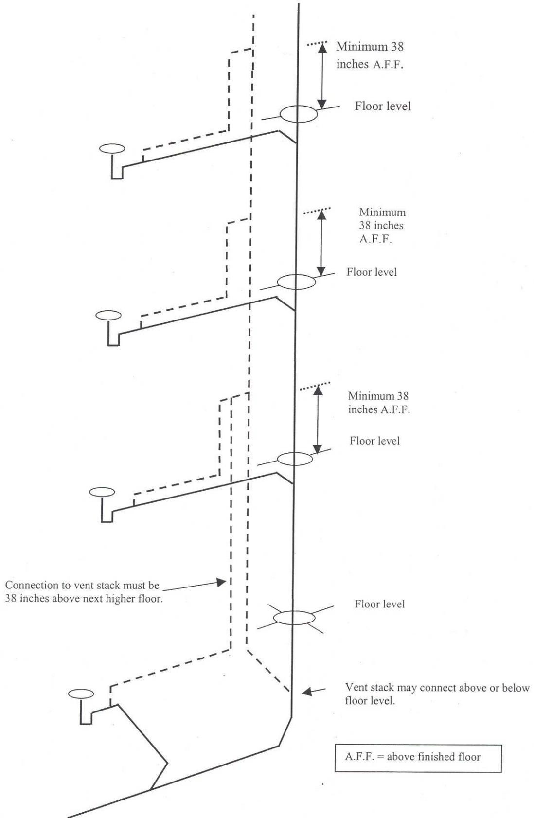
A-82.31 (4)-4. VENT STACKS AND STACK VENTS.
