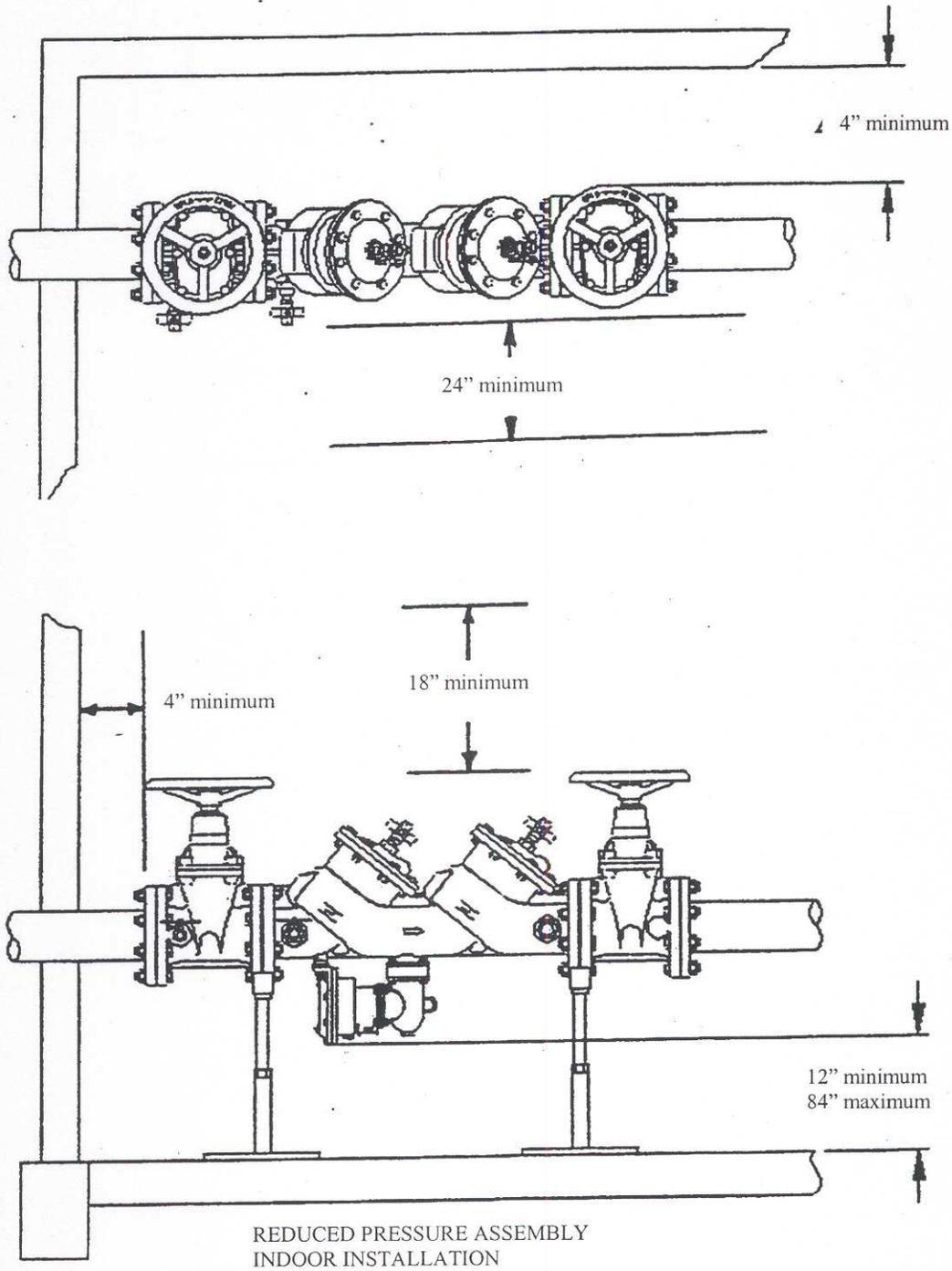
A-82.41 (5) (f)-2. CROSS CONNECTION CONTROL ASSEMBLY INSTALLATION.
