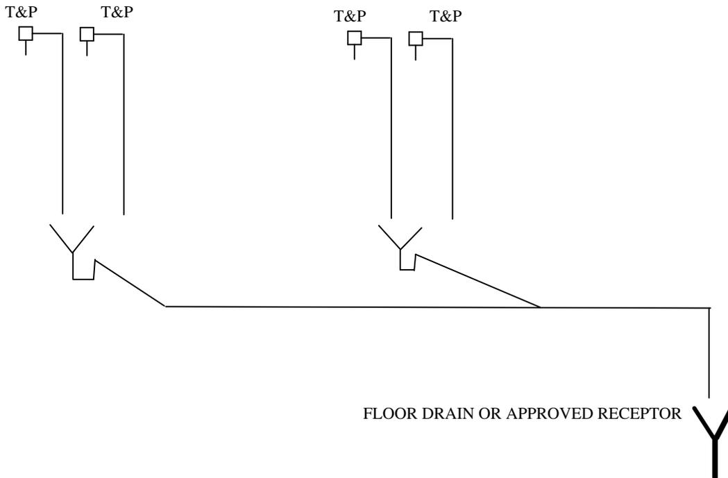
**A-82.33 (8) (d)-2. LOCAL WASTE PIPING SERVING WATER HEATER TEMPERATURE AND PRESSURE RELIEF VALVES.**
