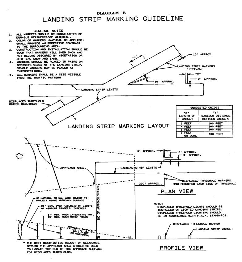
DISPLACED THRESHOLD MARKER LAYOUT
