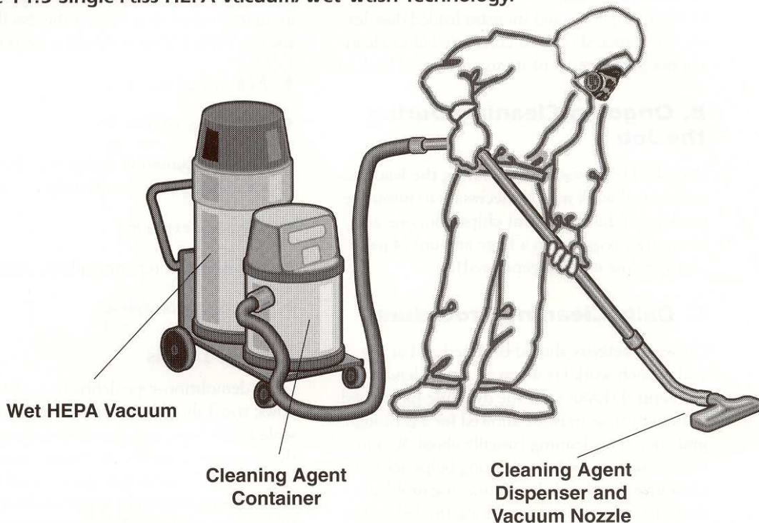
Figure 14.5 Single-Pass HEPA Vacuum/Wet Wash Technology.
