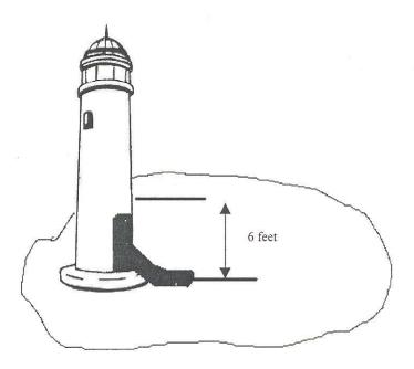
The square footage of the obstruction between the water level to a height of 6 feet for the obstruction shown is 48 square feet. This obstruction is code compliant, as provided in s. Comm 90.30, without a lifeguard staffing plan.
