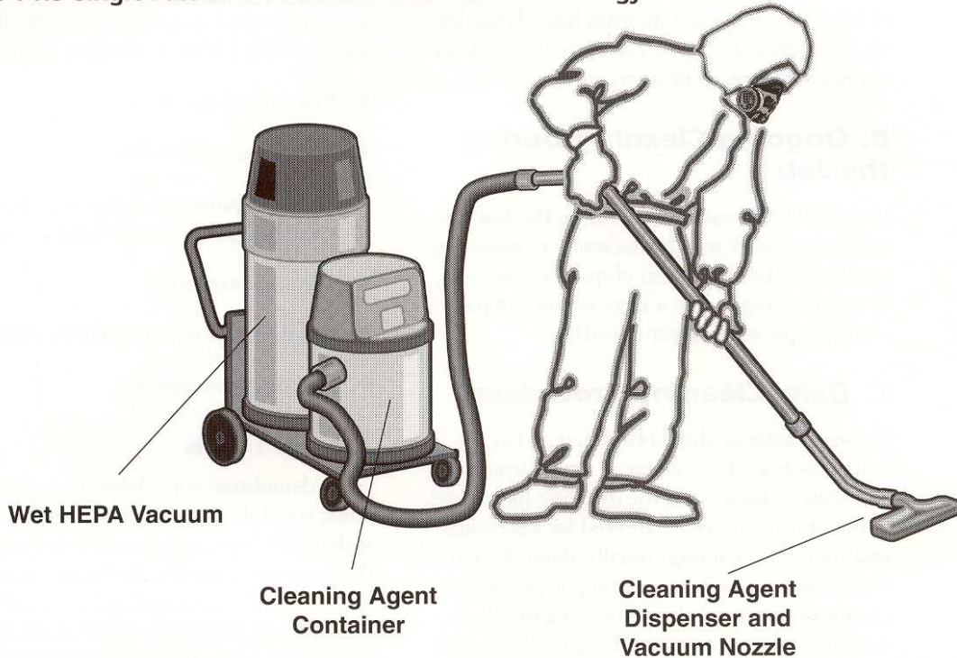
Figure 14.5 Single-Pass HEPA Vacuum/Wet Wash Technology.
