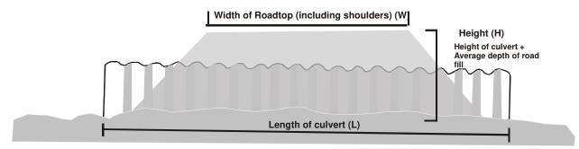
Determining the length of a culvert:
