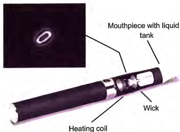
Fig. 1 Scheme of the tested e-cigarette A. The thermographic image shows the temperature distribution of the heating unit without 'liquid' ( > 350^{\circ}\text{C} in the center)
