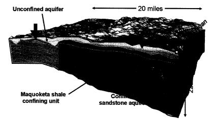
Figure 1. Hydrogeology of Southeastern Wisconsin. The confined aquifer in the graphic is the deep Aquifer. The blue arrows indicate direction of flow. The Maquoketa shale confines ground water below it and is a barrier to the flow of water to and from the surface. The dotted line is the surface water divide.
