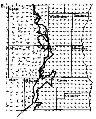
Figure 2. The St, Peter Aquifer groundwater divide (red line) under prepumping conditions relative to the western extent of the Maquoteka shale (black line) and flow of water in the aquifer (red – upward flow and blue – downward flow – arrows. Source: United States Geological Survey
