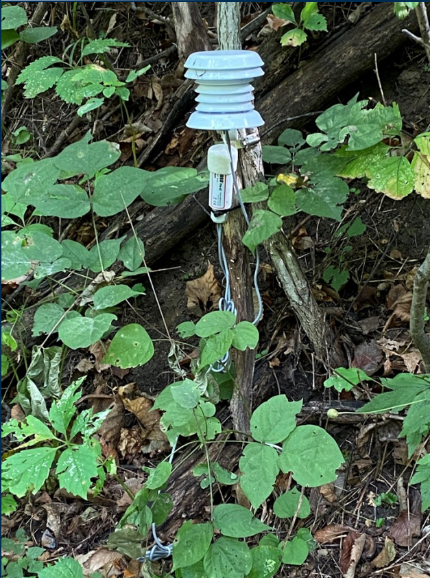
Data logger and solar radiation shield used to monitor Japanese stiltgrass in the Coulee Experimental State Forest. Photo Credit: Wisconsin DNR
